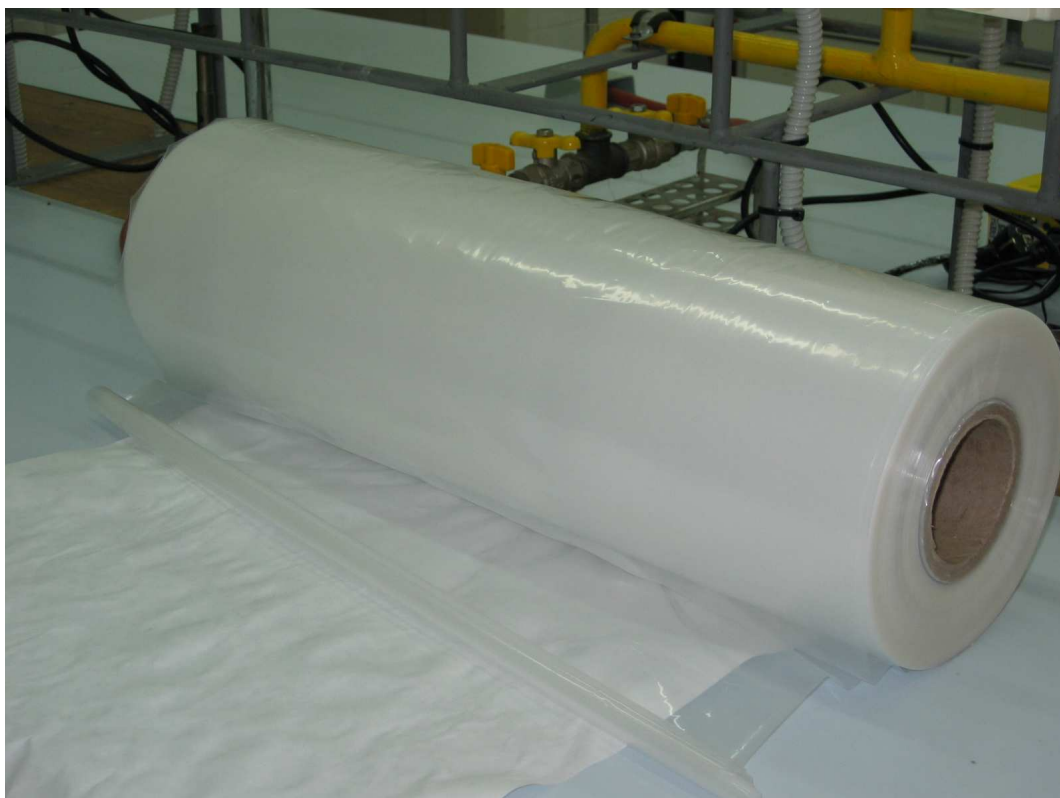
Figure 1 Packaging film INVOS II (type LDPE/PA, 78 \mu\text{m} , produced by INVOS a.s.) with both nisin and natamycin in lacquer layer (3 \mu\text{m} of Kombilack L-1471 containing 16.7 % (w/w) of Nisaplin and 33.4 % (w/w) of Delvocid)
