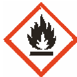
Danger Extremely flammable (liquid and vapour)
